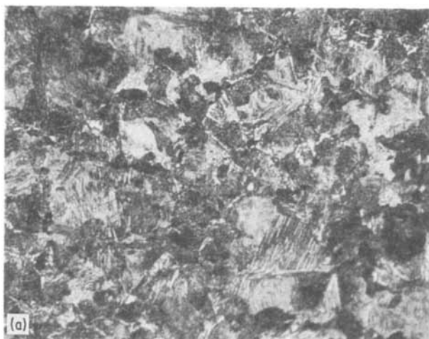
Figure 8 Microstructure of the 1045 steel sample quenched in SUNQUENCH 1032 at zero field, \times 546 . (a) 1 mm from the surface, (b) near the centre.
